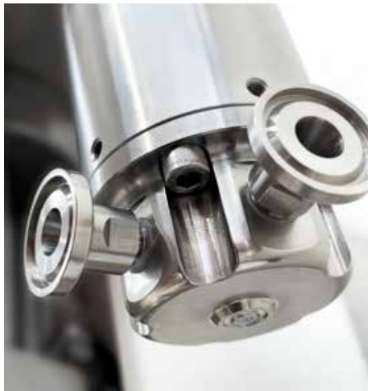
▼ MICRO DOSING HEAD FOR FILLING SUSPENSIONS AND SOLUTIONS
