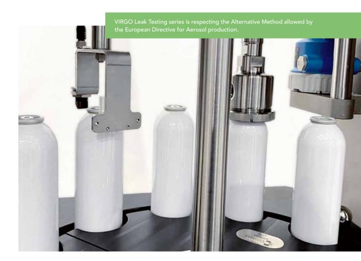
VIRGO is an electronic and programmable indexing machine available in both safe and ATEX execution configurations. The machine has been conceived to detect leakages in aerosol filling production lines due to defective valves.
