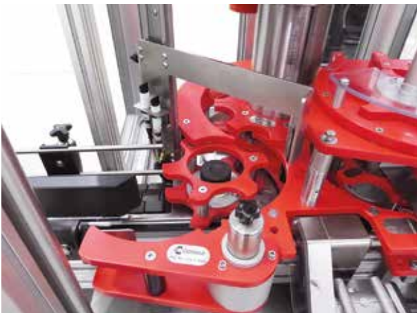
➤ CAP PLACING MACHINE WITH ELEVATOR
