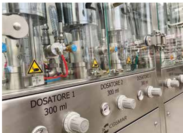
➤ PROPELLANT FILLING RACK
